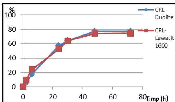
Fig. VIII.2. Thermal testing of (*l*)-butyrate of menthyl (45 °C)
